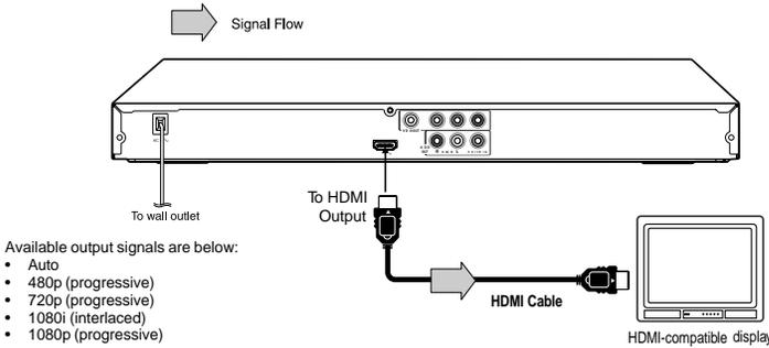
■ **Switching the video quality (HDMI mode) using HDMI button on the remote control or HDMI SELECT button on the front panel.**
