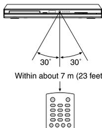
Distance: About 7 m (23 feet) from the front of the remote sensor
