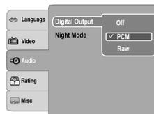
**PCM:** Select when connected to a Multi-channel digital stereo amplifier. The DVD player outputs sound in the PCM stereo format when you play a DVD recorded on the Dolby Digital, MPEG1 or MPEG2 recording system.
